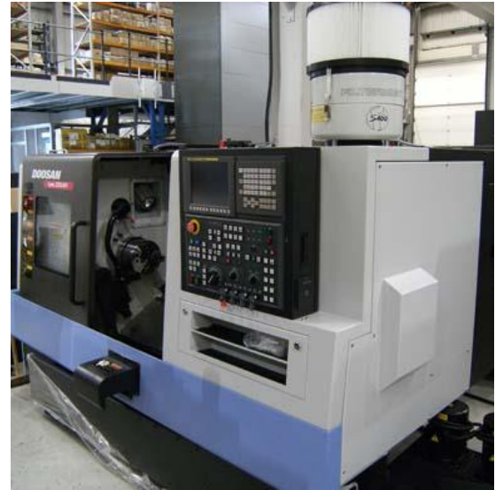
Filtermist Direct Mounted on Doosan Lynx
