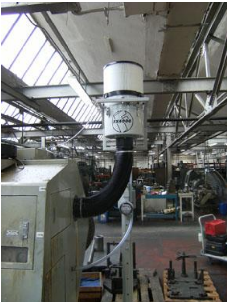
Filtermist Mounted on a Floor Stand Next to Nakamura Tome TMC35
