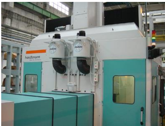
Two Filtermist Units Side Mounted on a Large Machining Center
