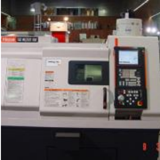
Filtermist Direct Mounted on Mazak Nexus
