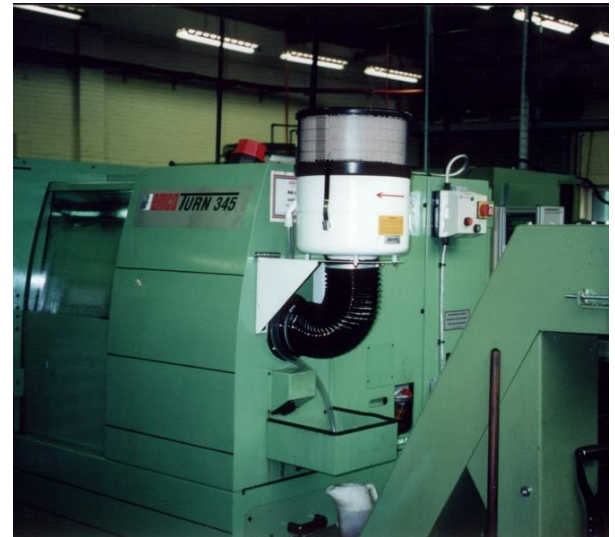
Side Mounting Bracket Used to Mount Filtermist on Emco Maier ET345
