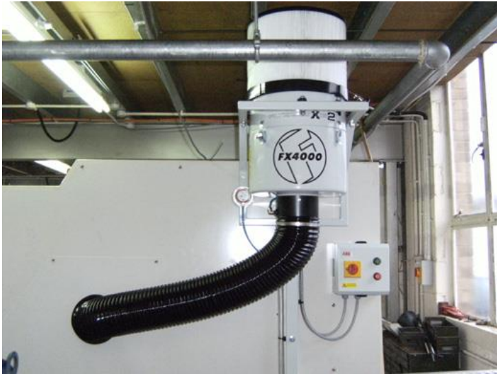
Filtermist Mounted with Side Mounting Bracket on Doosan Puma 200
