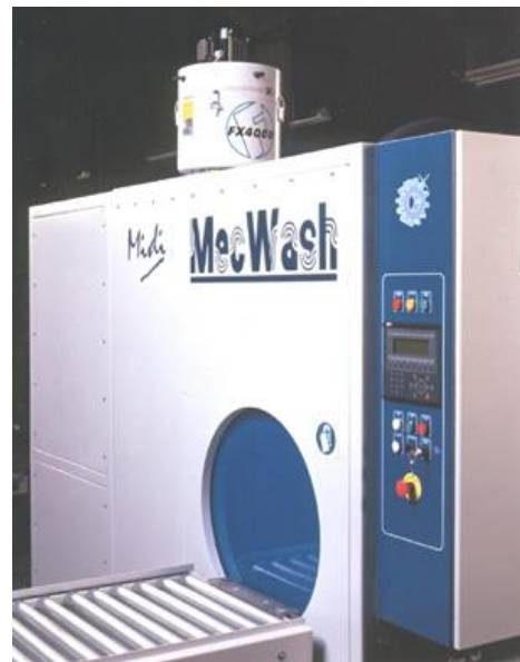
Filtermist Unit Mounted Directly on a Parts Washing Machine
