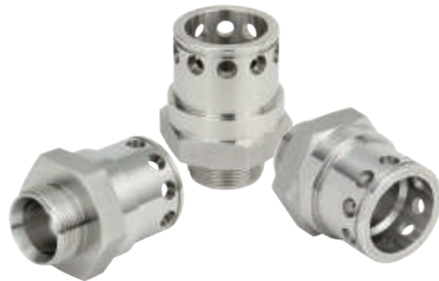
45x80mm - STAINLESS STEEL - HEX BAR STOCK CYCLE TIME: 16.5 SEC
