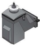
Included with the machine are four (4) CNC Rotary Tables. These tables are installed on stations 2, 3, 5, & 6 and have a position accuracy of +/- 4 seconds. Each table is equipped with a zero point clamping system, made by EROWA in Switzerland, to securely and accurately clamp the base pallet to the table. The positional repeatability of these pallets is less then 0.002 mm.
