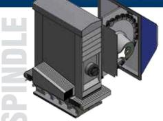
Each ICON 6-150 machining module is equipped with one (1) 42,000 RPM motor spindle. All spindles are a cartridge design and can be installed to any of the four (4) possible machine locations. They are air purged, liquid cooled and are permanently grease lubricated and therefore virtually maintenance free.
