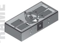
The Machine frame is designed as a sturdy, welded, steel construction. It supports the indexing table, the four (4) machining units as well as the B-tables. The openings below the machining stations assure an optimal evacuation of coolant and chips from the working area. Individually arranged and controllable coolant nozzles are installed inside of the machine frame for the purpose of providing coolant to the cutting tools and preventing chip accumulation inside the machining area.
