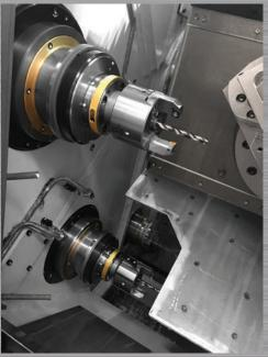
The 3-axis modules feature 20m/mm single lead ball screw assemblies, with the Z-Axis having a 180mm stroke while the X-Axis and Z-Axis both featuring a 60mm stroke each.
