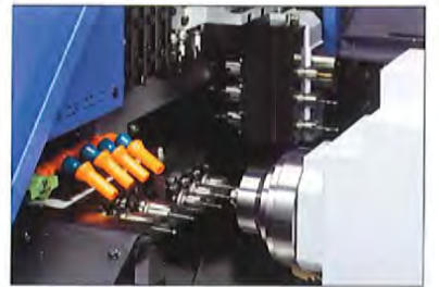
Back drilling by 3-spindle back drilling unit
