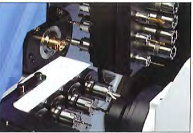
Front / rear-end simultaneous drilling
