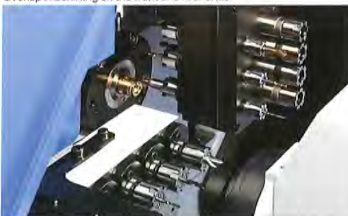
Overlap machining on the front and rear ends
