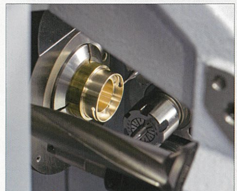
Cross hole ID chamfering
