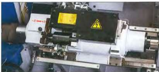
Main Spindle The headstock stroke of 350mm
