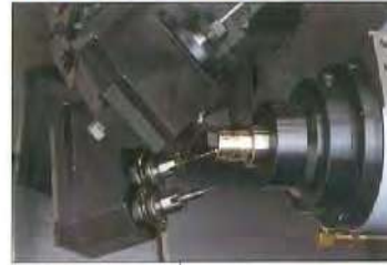
variation 01 Skewed Hole Drilling
