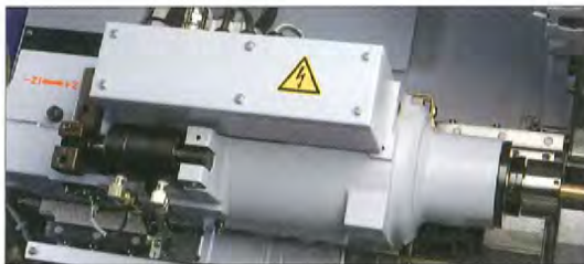
Machining bar materials of up to 350mm in length is possible with just one chucking.
