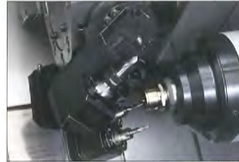
Skewed Hole Drilling
